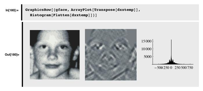
The determinant of the Hessian provides a simple measure of "salience" (See Torralba et al., 2006 for different model of salience, and an application to human vision.)
