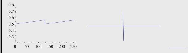
To handle gradients that aren't perfectly linear, we could add a threshold function to set small values to zero before reintegrating:
